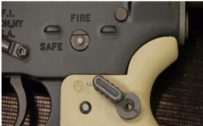
Most modern guns have one or more mechanical devices or subsystems designed to reduce the likelihood of an inadvertent discharge. These subsystems are collectively known as "safeties." Generally, safeties can be either "active" or "passive." Today, we'll cover active safety systems—those that are intentionally activated and deactivated by the user. (Passive safety systems work *without* your direct intervention.) Safeties are generally located on the
